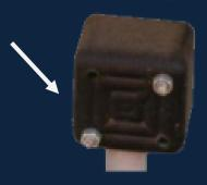
• Simple changes to the load cell mount and the use of only stainless steel for the base plates increases the longevity of the life of the weighbridge.
