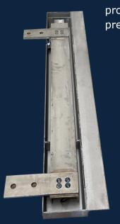
Load Cell are well protected from hole pressures
