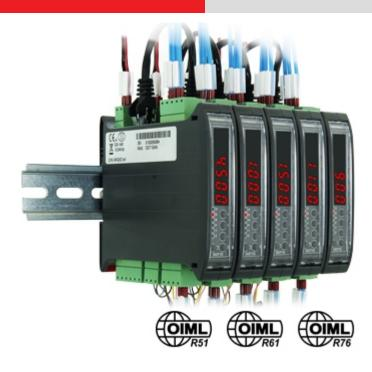
Compact, multifunction weight transmitter / indicator, for panel mounting on DIN bar. It allows the direct reading and diagnostics of the connected weighing system. The wide range of available interfaces, makes it easy to integrate the weighing with any automation system.
